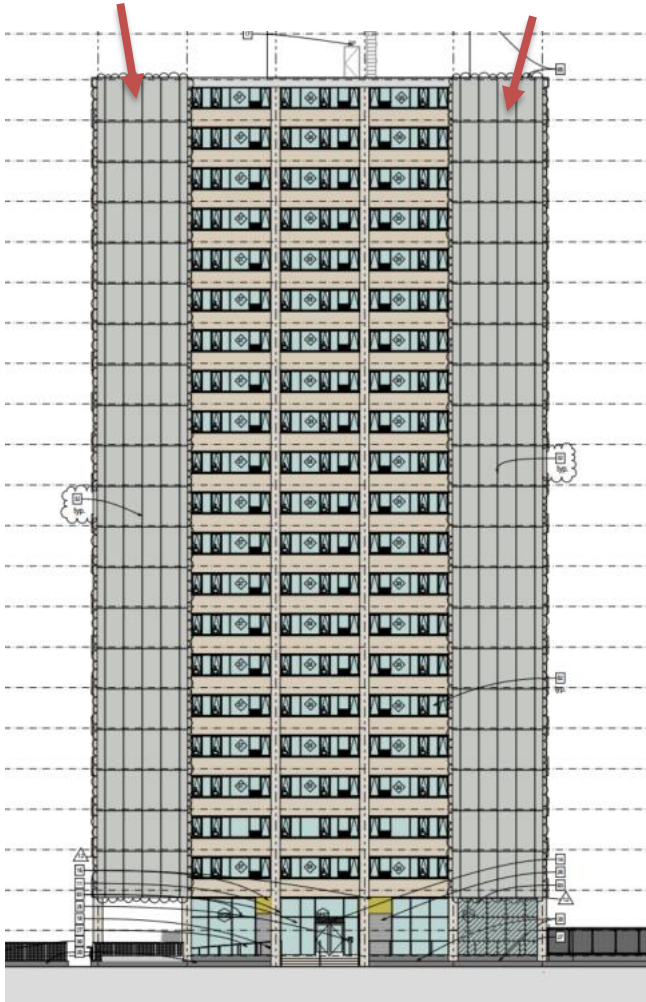
Full masonry wall rebuild (four corners) with steel framing and insulated panels
